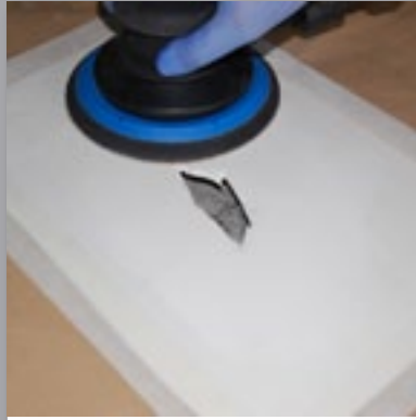
2 Remove all the loose/fractured particulate and paint from the affected area with a DA sander using a P80 grit disc.
