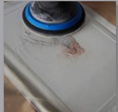
6 Once cured sand with a P40 or P80 to achieve general shape.
