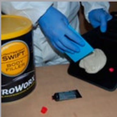
7 Once the area has been prepared mix your ProWorx filler with hardener at a ratio of 2% at an ambient temp of 20°C.
