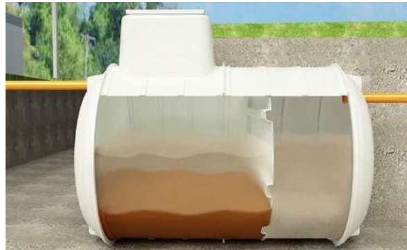
Domestic septic tank
